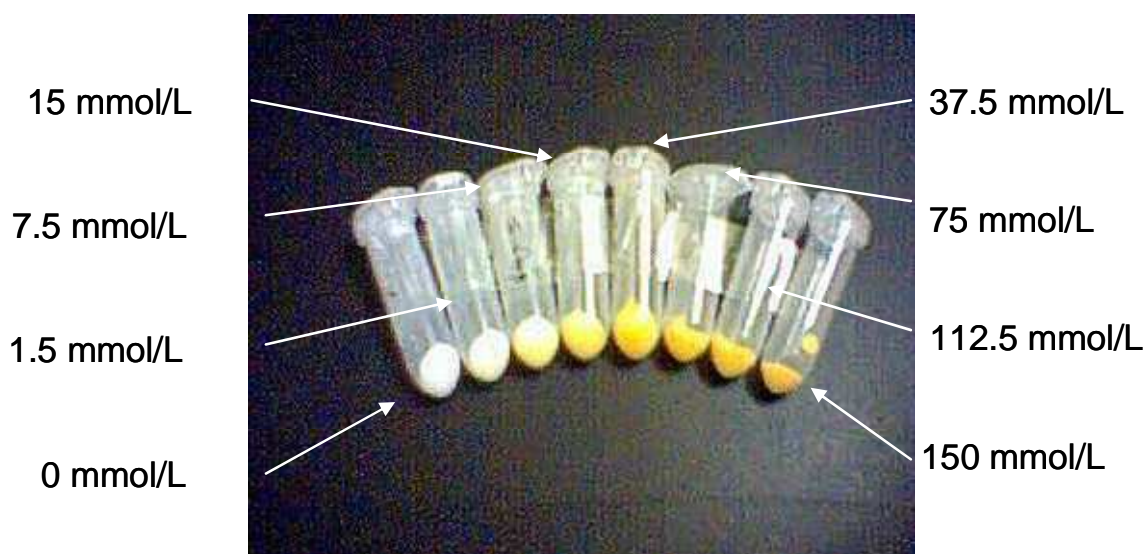
Fig. 2: TNBS-reaction performed after adsorption of pamidronate from solutions with different concentrations. From left to right the intensity of yellow color is strongly increased with rising amount of pamidronate indicating an increase in functional groups present on the surface.
