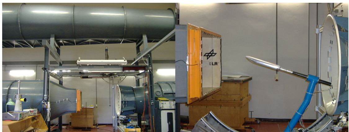
Figure 3.8. Left: the 1-meter low-speed open wind tunnel at the Institute of Aerodynamics and Flow Technology of the German Aerospace Center (DLR) in Göttingen. Right: the delta wing attached on the angle transmitter and mounted in the measurement section of the wind tunnel.
