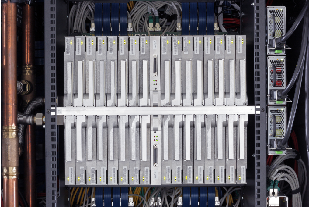
Figure 2.1: Photo of a fully populated QPACE Cold-Plate. The plate is in the very center of the picture. There are 32 Node Cards as well as 2 Root Cards attached to it. On the left one can see the piping that provides cold water to the Cold Plates. On the right there are three power supplies, one for redundancy.
