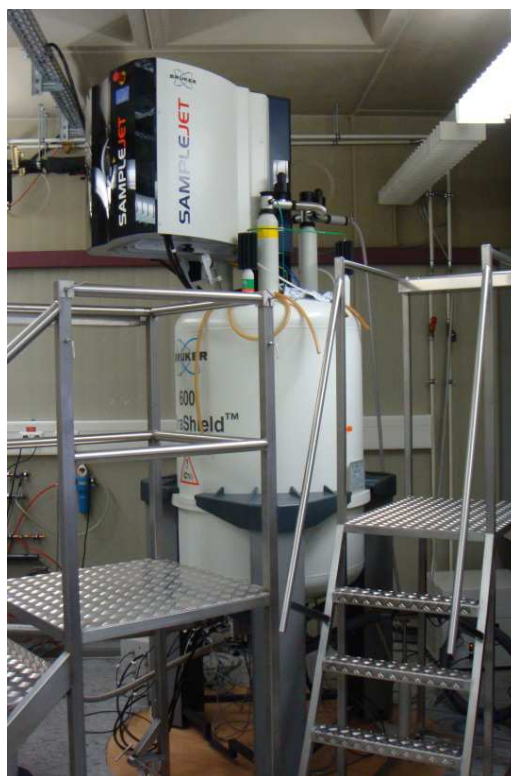
Figure 7. The 600 MHz Avance III cryo probe spectrometer with a cooled automatic sample changer was used for all NMR measurements in this thesis.
