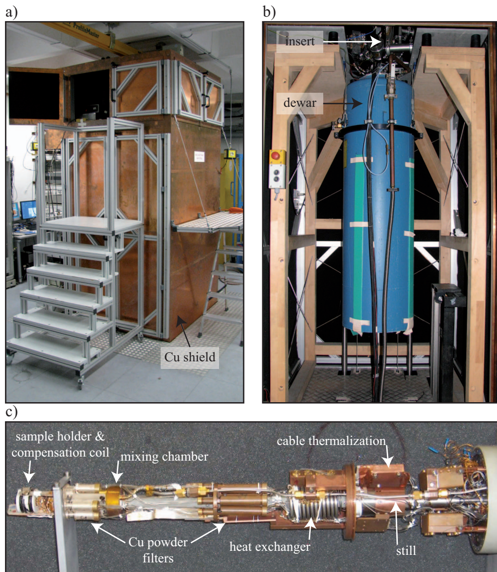
Figure 5.7.: Photographs showing different views of the dilution refrigerator measurement setup. (a) Overview, showing the copper shield which completely surrounds the low temperature part. (b) Dewar with the dilution system inserted. (c) Dilution system without vacuum shields.
