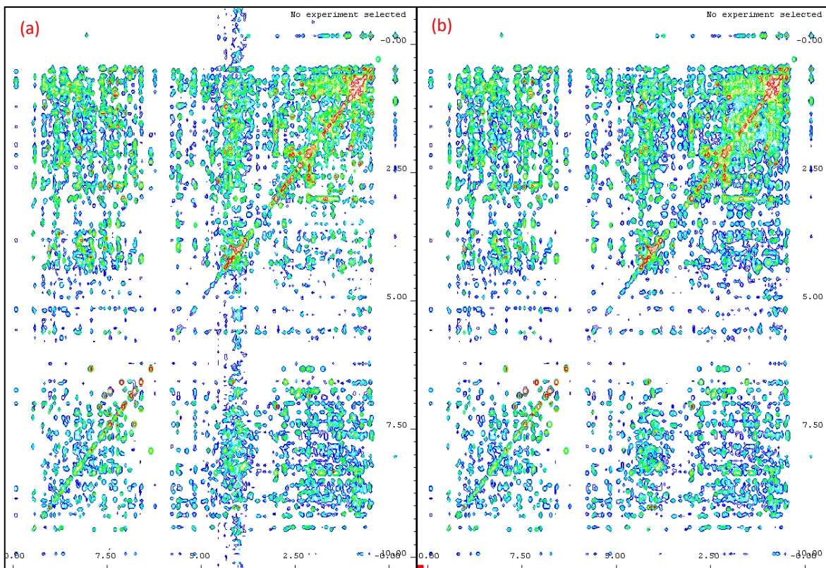
Figure 3.6 SSA of a back-calculated spectrum without solvent: a simulated two-dimensional spectrum (par. 2.1.1.1) of HPr from Staphylococcus aureus (H15A) after (a) and before (b) SSA. The experimental solvent signal has not been added to the protein spectrum, thus the SSA automatically removes some resonances of the solute, generating spectral distortions.
