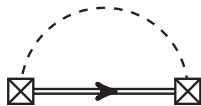
FIG. 2. Impurity-averaged self-energy which determines the Elliott-Yafet collision operator. The boxed crosses, the dashed line, and the arrowed double line represent spin-orbit coupling, impurity correlations, and the Green's function in Keldysh space, respectively.
