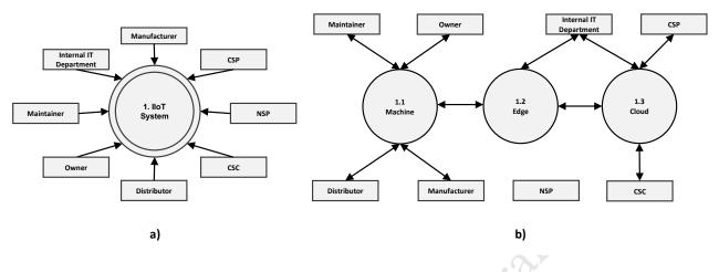
Figure 2: context diagram on level-0 (a) and data flow model on level-1 (b).
