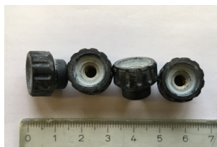
Figure 12: The locking nuts required to lock the beakers into place with metal plates.
