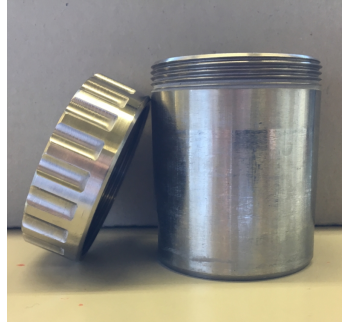
Figure 14: A 100 mL stainless steel beaker used to for the samples tested in the DTU.
