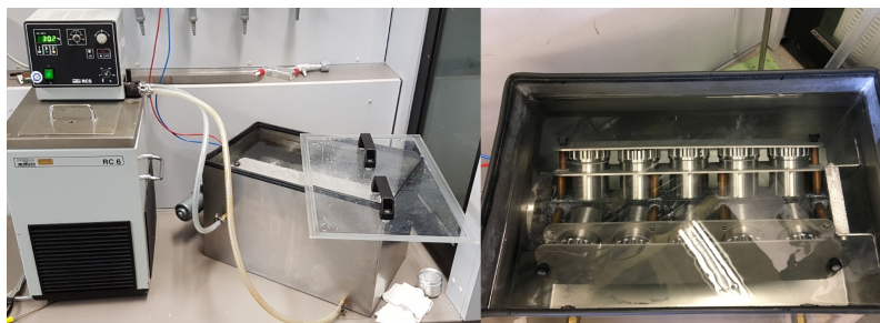
Figure 9.2: Left: complete DTU with a standard laboratory cryostat connected. Right: View inside the container with the axis being fully mounted with beakers.
