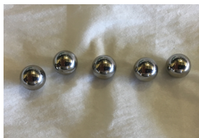
Figure 15: The 8 mm stainless steel balls used to simulate mechanical input in laundry washing processes.
