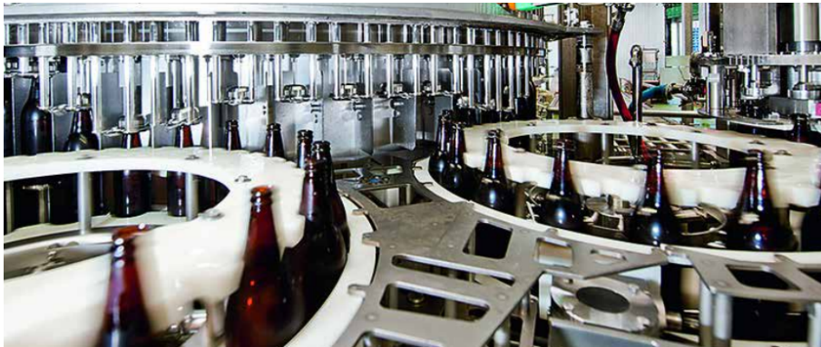
Figure 6.5: Example of two transfer stars (white) transporting the bottle to and away from the big filler carousel in the middle.[67]
