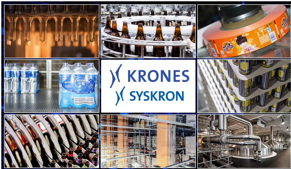
Figure 1.1: Overview over different Krones machines, clockwise from top left: Blower, Filler, Labeller, Palletizer, Brew House, Warehouse, Bottle Washer and Packer.[68]
