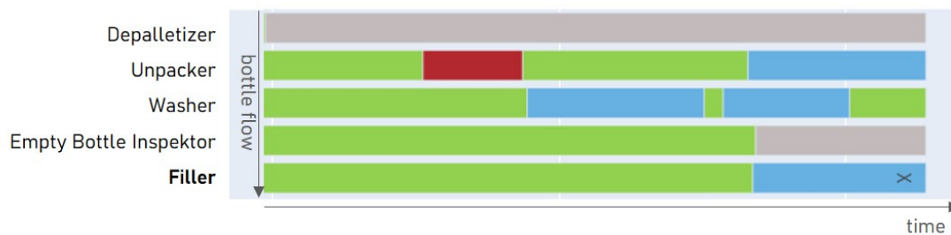
Figure 4.2 Gantt chart showing wrong machine state of EBI at customer-a in case of lack from Depalletizer. Thus EBI should show machine-state "lack" when stopping as a cause of Depalletizer error. Production is displayed in green, "tailback" in pink, "lack" in blue, and "held" and "off" in grey. "held" and "off" are own-fault states of the machines.
