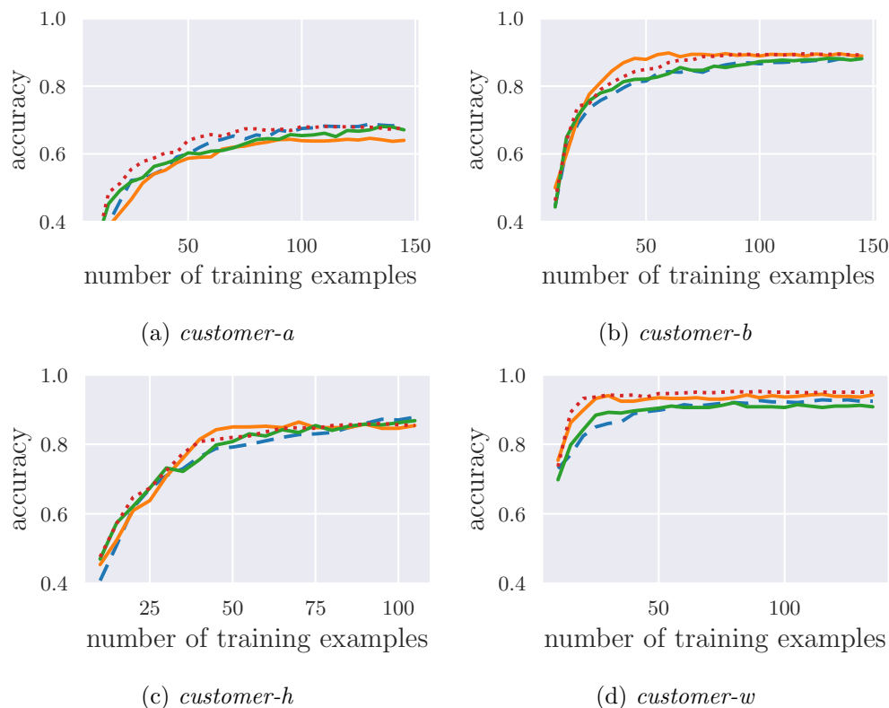
Figure 4.26 Comparing different query strategies for pool-based Active Learning. AL starts with 10 labeled samples. Model: Random Forest with 500 estimators and maximum depth of 7. Training is conducted for every number of training samples 10 times and results are averaged. Random Sampling strategy is plotted in dashed blue, Uncertainty Sampling in orange, Nearest Neighbor Criterion in green and Dynamic Ensemble Active Learning in dotted red.
