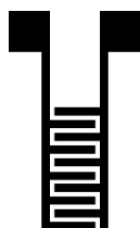
SI Figure 3.10 Layout of an interdigitated Laser-Induced-Graphene electrode on polyimide substrate
