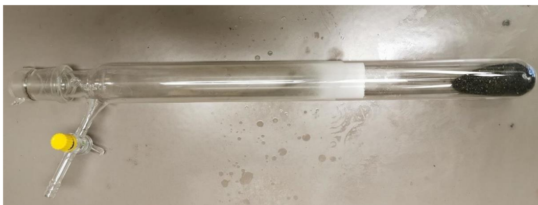
Figure 2.1.1: Purification of arsenic: Purchased arsenic was purified by sublimation in a Schlenk tube – pure arsenic is seen on the right-hand side while sublimated \text{As}_2\text{O}_3 is seen on the left-hand side.
