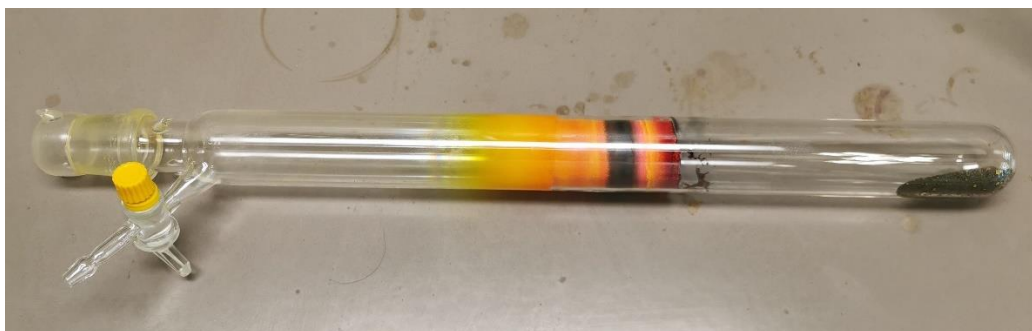
Figure 2.1.2: Sublimation of melt of realgar (As 4 S 4 ) to yield pure realgar crystals (seen as bright yellow on the left-hand side of the Schlenk tube).
