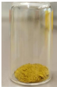
Figure 3.2.1.1: Phase pure yellow (AgI) 2 ·(As 4 S 4 ) synthesized via solid state route.
