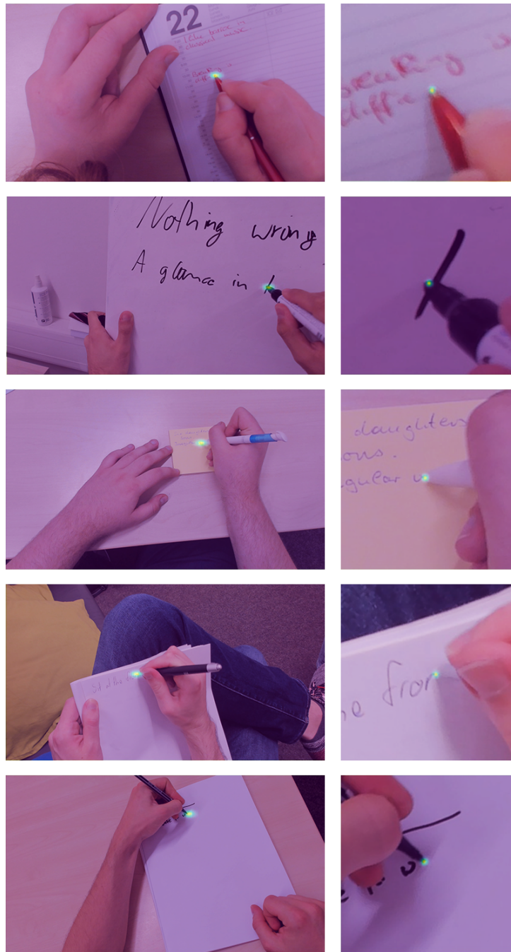
Figure 8.1. – Frames from the test set of POV-Keypoint and the resulting heatmaps produced by the ResNet-50-L-NF keypoint detection variant, where bright green means high certainty. The images on the left show the output of the ROI detection network overlaid on input frames. The images on the right show the image patch extracted using ROI peak detection with the detail tip detection laid over it.
