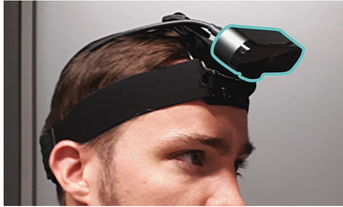
Figure 6.1. – The head mounted camera setup, using a Logitech BRIO Webcam.
