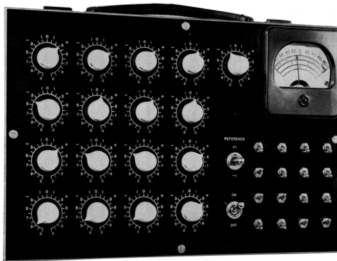
Figure 5.2. – ADALINE: One of the early artificial neural network machines (Widrow, 1960).
