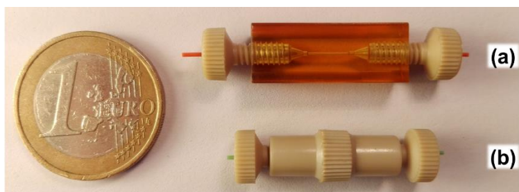
Figure D.3. Photograph of the transparent, laboratory-constructed capillary connector fabricated from polyetherimide (a) and the commercially available capillary connector fabricated from polyether ether ketone (b)
