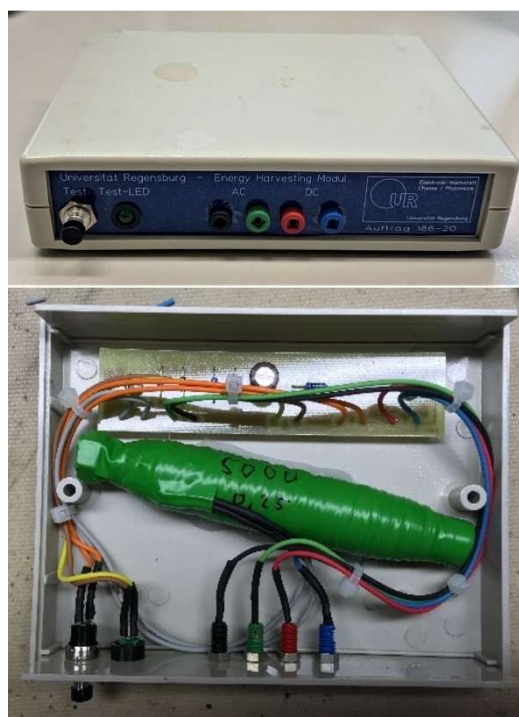
Figure S 1. EH device. top: front view, bottom: view into the opened housing.
