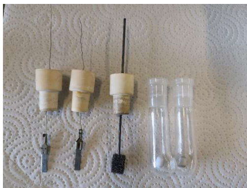
Figure S 1. Electrodes and H cell setup: Zn-electrode (left), steel-electrode (center), RVC-electrode (right).
