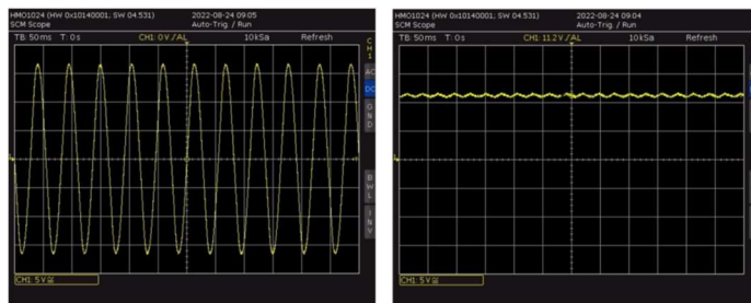
Figure 2. Oscillogram of the output voltage of the EH device. Left: open circuit without rectification, right: closed circuit under load with rectification.
