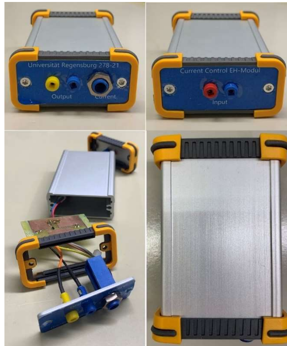
Figure S 4. Current control module. Top: front and back view, bottom: opened and closed housing.
