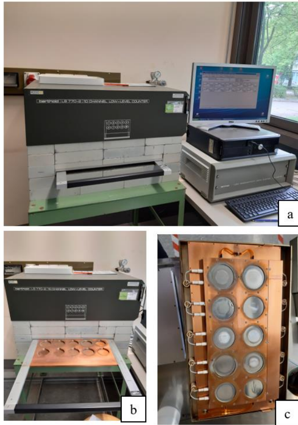
Figure 16: Real depiction of the LB 770-2Win-PC 10 channel measuring station a) complete device with detector, interface, gas supply and computer b) an extendable slide for the 10 measurement trays c) flow-meter set-up installed over the measurement sites
