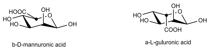
Figure 21: \beta -D-mannuronic acid and \alpha -L-guluronic acid in their {}^4C_1 conformation; the black dot marks the stereogenic center, which differs in the two epimers; guluronic acid is not in its more stable {}^1C_4 conformation, as the carboxylic acid group is in an unfavorable axial position.
