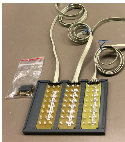
Figure 65. A photo of the 96-well plate LED lid, featuring exchangeable LED boards of a specific wavelength that allow for irradiation of 72 individual wells in a 96-well plate.
