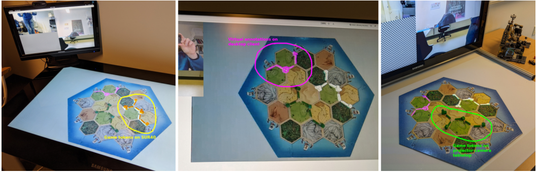
Fig. 5. SurfaceCast running on three clients while playing a board game (Settlers of Catan). Left: a SUR40 tabletop with physical yellow tokens; center: a desktop client using virtual magenta-coloured annotations; right: a SurfaceStation device with physical dark-green tokens and physical game board. For each client, the local components are circled in the corresponding color. The "front mosaic" is visible in the background screens on the left and right clients.
