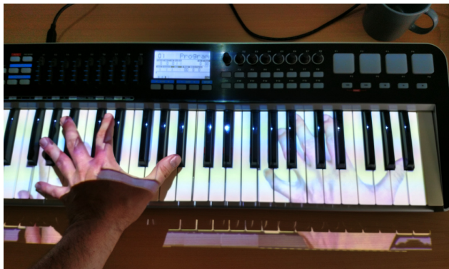
Fig. 10. Piano teaching scenario. The projected hand of the teacher is visible on the right, while the student emulates the pose with their own hand on the left.
