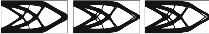
Fig. 4 Numerical results for joint optimization of compliance and principal eigenvalue with weight \alpha \in \{10, 100, 500\} (left to right). We observe that increasing the weight \alpha of the first eigenvalue leads locally to a finer structure
