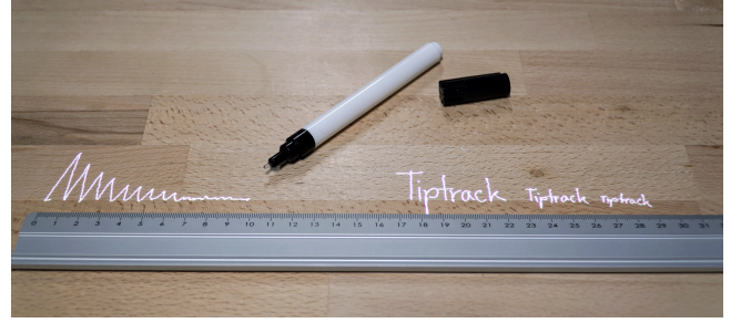
Figure 10: Text written with TipTrack remains readable up to a minimum letter height of approximately 4 mm.
