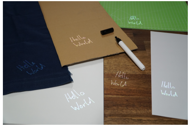
Figure 6: TipTrack can reliably track the infrared pen on different flat and smooth surfaces, such as paper, cardboard, wood, and fabric.
