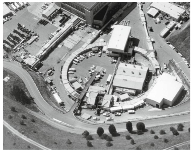
Fig. 4 The 80m SPEAR Ring in a parking lot at SLAC. The photo also shows the separate e^+ and e^- beam lines and the detector hall
