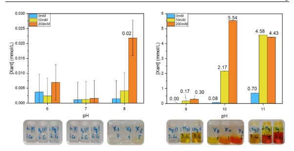
Figure I.30. Maximum solubility of xanthohumol as a function of pH and meglumine concentration. Blue: ultrapure water (no meglumine). Yellow: 50 mM meglumine in ultrapure water. Orange: 200 mM meglumine in ultrapure water. The results are shown in two different graphs to adapt the scale of the xanthohumol concentration axis.
