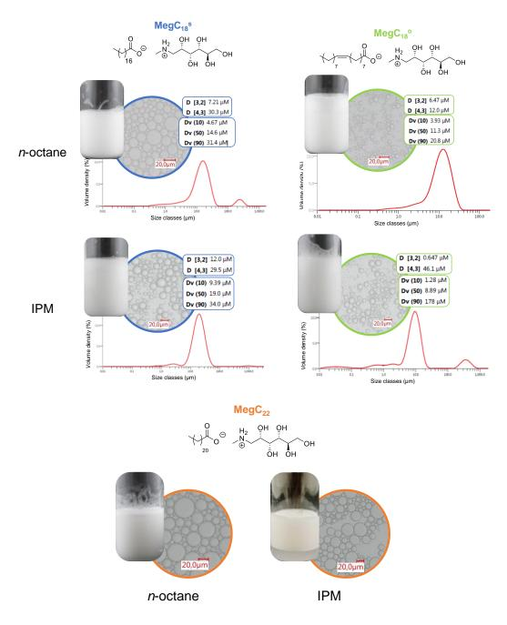
Figure IV.20. Macroscopic and microscopic pictures of n-octane/water and IPM/water emulsions from  $MegC_{18}^{s}$ ,  $MegC_{18}^{o}$ , and  $MegC_{22}$ , as well as granulometry analysis for  $MegC_{18}^{s}$  and  $MegC_{18}^{o}$  emulsions. Emulsions prepared according to protocol 1.
