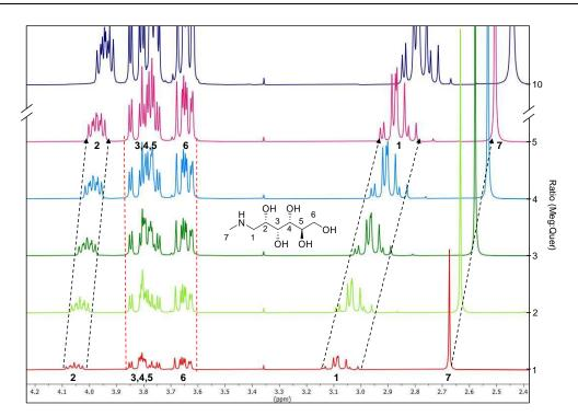
Figure I.24. <sup>1</sup>H NMR spectra of meglumine (Meg) in the presence of quercetin (Quer) in D<sub>2</sub>O at increasing meglumine to quercetin molar ratios from bottom (1:1) to top (10:1). Dotted lines serve as visual guides for the evolution of the chemical shifts.
