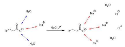
Figure IV.5. Representation of the charge screening of an anionic surfactant by increasing the ionic strength. Example of a carboxylate with increasing sodium chloride concentration.
