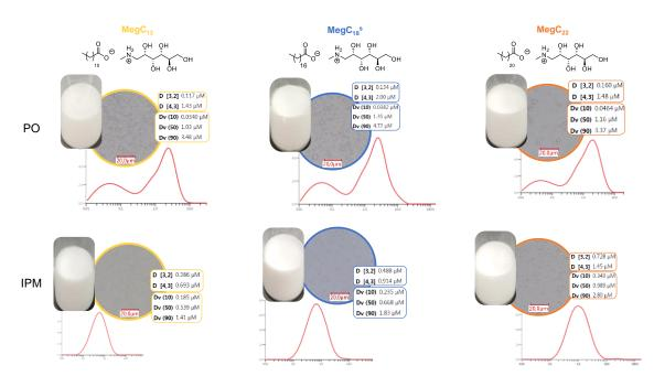
Figure IV.22. Macroscopic, microscopic pictures, and granulometry analysis of PO/water and IPM/water emulsions from MegC<sub>12</sub>, MegC<sub>18</sub><sup>s</sup> and MegC<sub>22</sub>. Emulsions prepared according to protocol 2.
