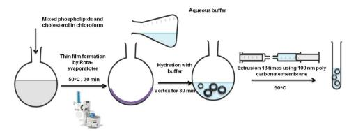
Figure II.2. Thin-film extrusion method. Reproduced with permission from reference [<sup>133</sup>].
