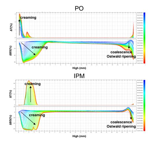
Figure IV.23.  $\Delta T$  and  $\Delta BS$  signals evolution for MegC<sub>12</sub> PO/water (top) and IPM/water emulsions prepared according to protocol 2.
