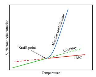
Figure IV.3. Schematic representation of the relation between surfactant solubility, CMC, and Krafft point. Based on reference [<sup>210</sup>].
