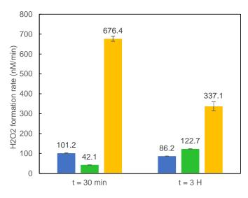
Figure I.28. Temporal evolution of H<sub>2</sub>O<sub>2</sub> formation rate of 0.1 mM quercetin samples in aqueous solution at pH 8. Blue: quercetin alone. Green: (100:1) meglumine-to-quercetin. Yellow: (1000:1) meglumine-to-quercetin.
