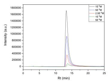
Figure A.1. Quercetin pure samples in MeOH for establishing the calibration curve of area under the curve versus quercetin concentration.
