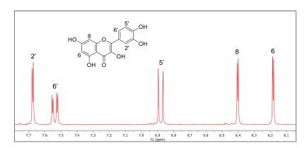
Figure I.22. <sup>1</sup>H NMR spectrum of pure quercetin in DMSO-d<sub>6</sub>.
