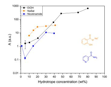
Figure III.12. Solubilization profiles in water of quercetin with ethanol (black), sodium salicylate (orange), and nicotinamide (blue).
