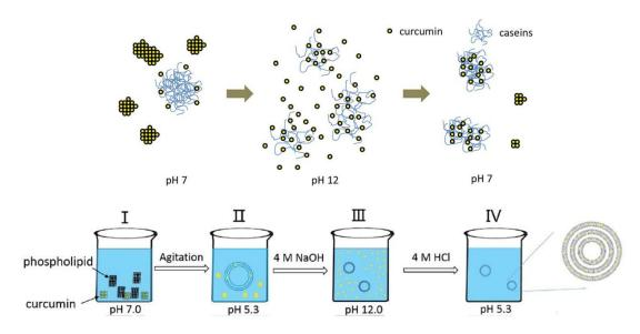
Figure II.3. Top: principle of the first pH-driven method for encapsulating curcumin into caseinate structures. Reproduced with permission from reference [<sup>129</sup>]. Bottom: application of the pH-driven method for encapsulation of curcumin into liposomes. Reproduced with persmission from reference [<sup>141</sup>].
