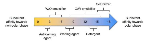
Figure IV.4. Representation of HLB scale and associated applications for surfactants.
