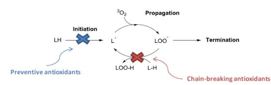
Figure I.7. Mechanisms of inhibition of oil oxidation by primary and secondary antioxidants. Reproduced with permission from reference [<sup>47</sup>].
