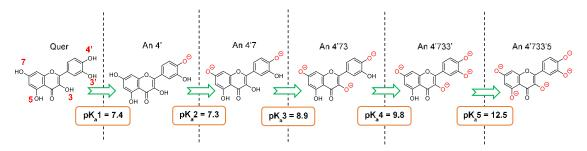
Figure V.2. pK<sub>a</sub> calculations for the most probable deprotonation order of quercetin according to the COSMO-RS method.
