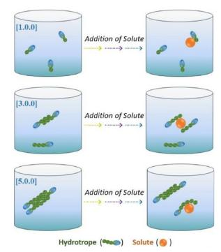
Figure III.3. Schematic representation of the hydrotropy mechanism with varying degrees of hydrophobicities. Reproduced with permission from reference [<sup>157</sup>].
