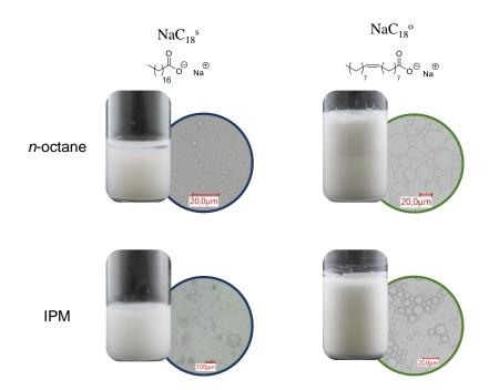
Figure IV.21. Macroscopic and microscopic pictures of NaC<sub>18</sub><sup>s</sup> and NaC<sub>18</sub><sup>o</sup> n-octane/water and IPM/water emulsions. Emulsions prepared according to protocol 1.
