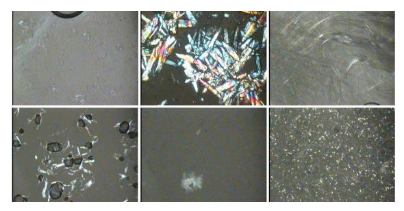
Figure A.6. Polarized micrographic pictures of  $GuC_{16}$  (top left),  $mGuC_{16}$  (top center),  $MetC_{16}$  (top right),  $GuC_{18}$  (bottom left),  $mGuC_{18}$  (bottom center), and  $MetC_{18}$  (bottom right) at 20°C. Magnification x100.
