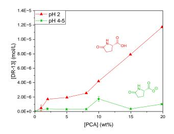
Figure III.15. Solubilization profiles of DR-13 with L-pyroglutamic acid (PCA) at two different pH values. pK<sub>a</sub> of PCA was experimentally determined at 3.3 (see Figure A.5 in Appendix A.5).
