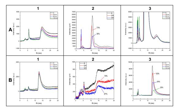
Figure I.26. Chromatograms for the temporal monitoring of quercetin oxidative degradation. **A**. In the presence of meglumine. **B**. With NaOH. **1**. At pH 7.35. **2**. At pH 8.4. **3**. At pH 11. All spectra were recorded at  $\lambda = 370$  nm. Percentages expressed represent the amount of unaltered quercetin.
