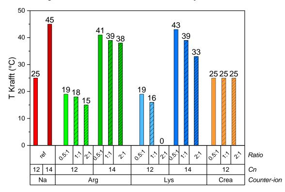
Figure IV.19. Screening of the influence of the addition of amino-acids on the Krafft temperature of sodium soaps. Arg refers to arginine, Lys to lysine, and Crea to creatine. Ratios represented are the amino-acids-to-carboxylate ratios.
