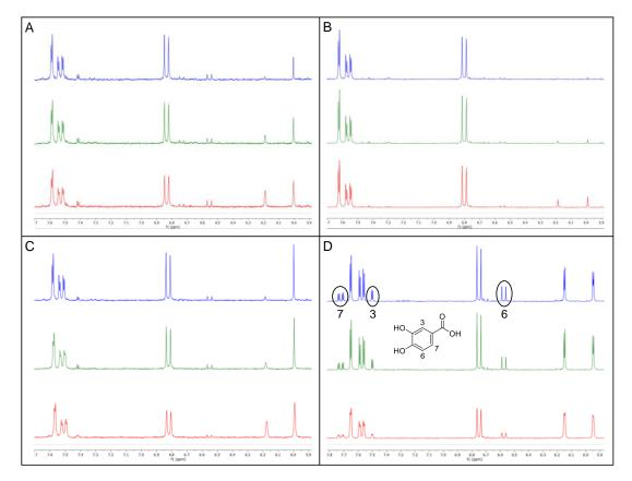
Figure I.25. 1H NMR spectra of quercetin in aqueous solutions in D2O over time. A. Meglumine to quercetin molar ratio of (1:1) (pH = 9.0). B. Meglumine to quercetin molar ratio of (5:1) (pH = 10.0). C. NaOH to quercetin molar ratio of (1:1). D. NaOH to quercetin moar ratio of (5:1).
