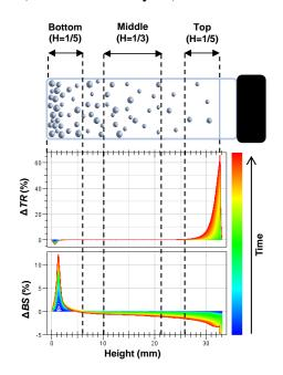
Figure IV.13. Representation of the evolution of transmitted  $\Delta TR$  and backscattered light  $\Delta BS$  measured with Turbiscan® for a partially sedimented dispersion. Reproduced with permission from reference [<sup>257</sup>].
