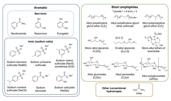
Figure III.4. Chemical structures of main hydrotropes classes.
