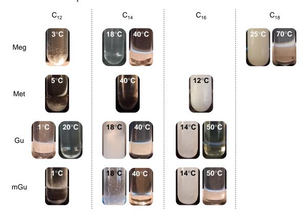
Figure IV.17. Photographs of Meg-, Met-, Gu-, and mGuC<sub>12-16</sub> at different temperatures. Gu- and mGuC<sub>14</sub> and Gu- and mGuC<sub>16</sub> are very viscous above 40°C and 50°C, respectively.
