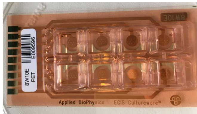
Figure 4.20 Image of an 8W10E array used for ECIS experiments with eight wells each having ten small WEs ( d = 250\text{ }\mu\text{m} each, total WE area A \approx 4.9 \cdot 10^{-3}\text{ cm}^2 ) with one common CE in the middle of the array reaching into each well. Nine contact pads served for electrical connection of the electrodes (eight WEs and one common CE) to the measurement device. Substrate and wells were made of PET and electrodes were made of gold. Electrical insulation of electrical supply lines was achieved by photopolymer coating.
