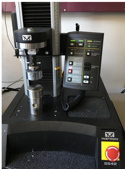
Figure 4.7 Material testing system Instron 5542 used for the determination of the Young's modulus E of PAAm gels A – E by compression testing. Cylindrical hydrogels were placed onto the fixed lower plate after their polymerization and compressed by the movement of the upper plate.
