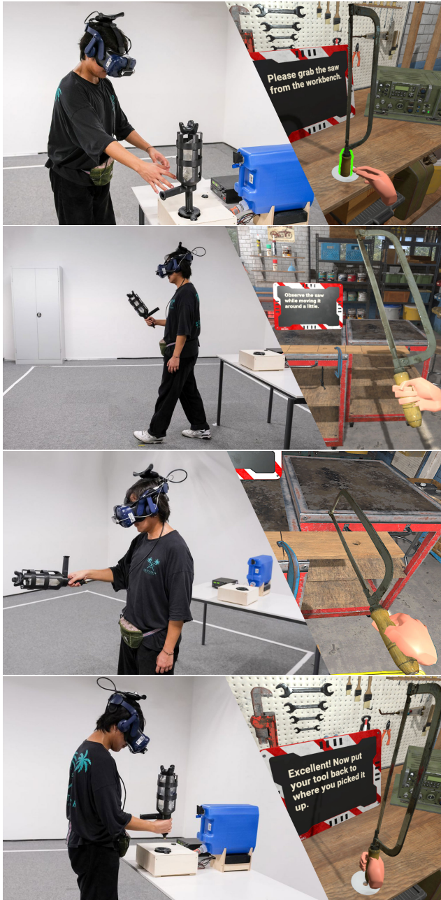
Figure 6: User picking up a virtual saw (top row), familiarizing himself with the saw (second row), working on the bird house with it (third row), and returning it (bottom row).
