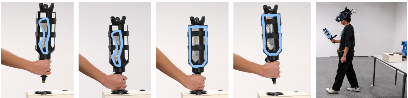
Figure 1: Procedure for adjusting the perceived weight through MobileGravity. The four images on the left show connecting MobileGravity's handheld proxy object with its base station, adjusting its weight, and disconnecting both components. The user can then move around freely (image on the right). The outline of the liquid reservoir inside the proxy object is highlighted.
