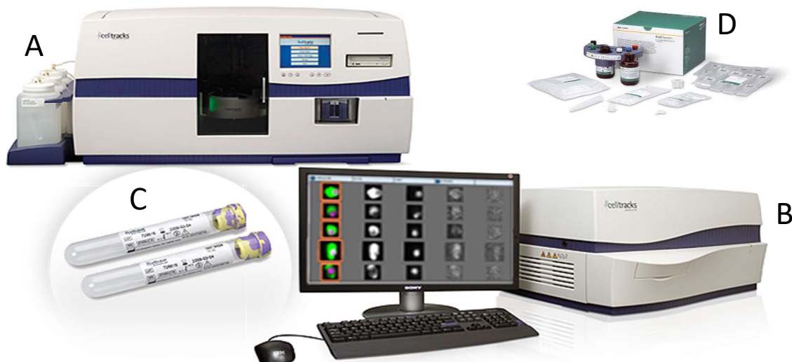
Figure 1 The CellSearch™ System with its compartments. The CellTracks® Autoprep (A) and the CellTrack® Analyzer II (B). For analyzing the samples the CellSave Tubes (C) and an appropriate Kit, in this case the CellSearch™ Circulating Tumor Cell Kit (D) are required. https://www.cellsearchctc.com
