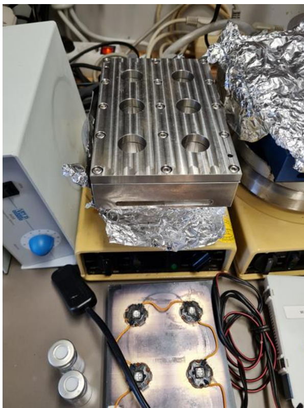
Figure S4.1. Thermostated metal block for simultaneous irradiation of 6 reaction vials.
