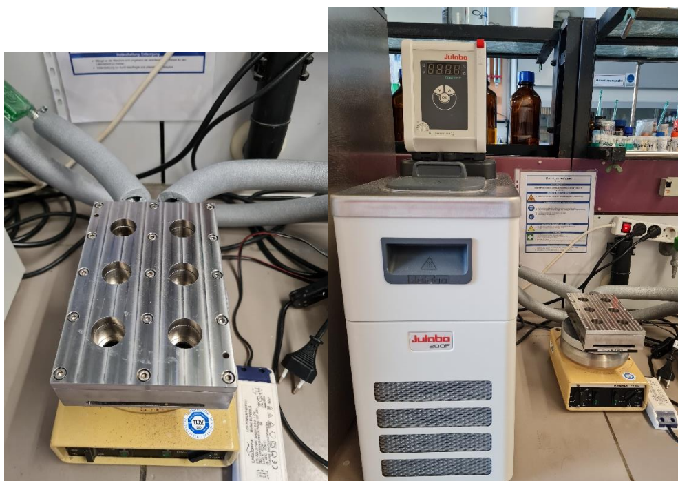
Figure F5.2. Cooling block and cryostat for the photoreactions at 4 °C.
