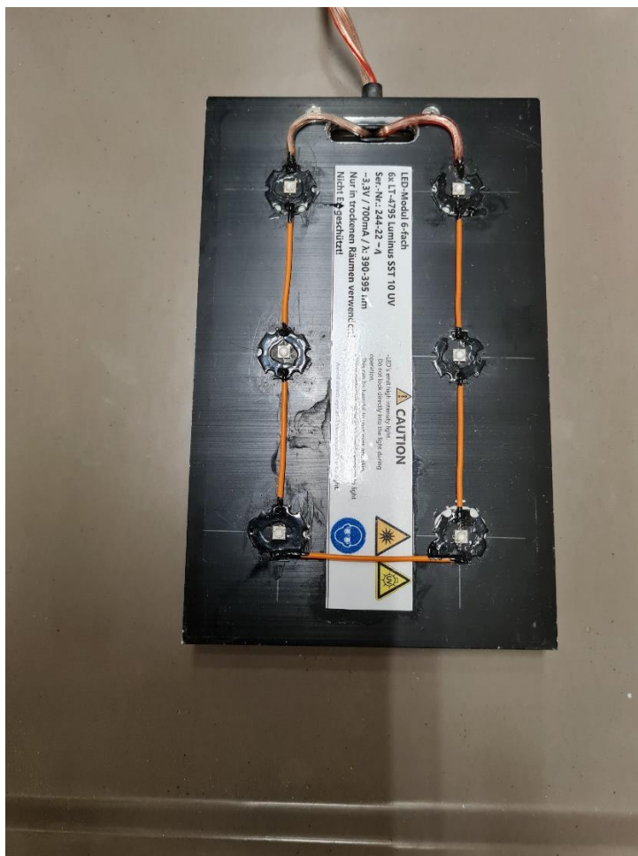
Figure S3.2. LED plate for the irradiation of six samples at the same time at 390-395 nm.
