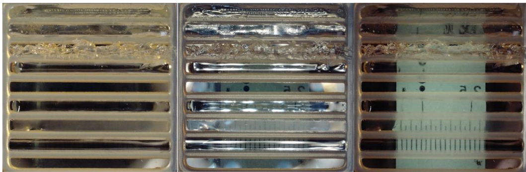
Figure 2.19: A prism was equipped with a silicone grid. Various adhesives were applied to this grid. On the left with reflected light, in the middle with reflected light and transmitted light, on the right with transmitted light.
