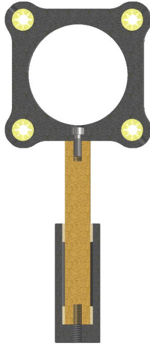
Figure 2.5: Corner Joint. The base of the corner joint can be attached to the base plate provided for the SPR measuring device using an M6 thread in the base and a grub screw to DIN 914. Two plain bearings are pressed into the base. These enable the joint post to be mounted without play and with low friction. The base is made of black anodized aluminum to minimize reflections. The post, on the other hand, is made of polished brass to achieve the best possible gliding properties. A mounting plate suitable for the respective cage system is mounted on the post using a burnished M4 screw to DIN 912. Plain bearings (igus RJMP-01) are pressed into the mounting plate. These enable the optical bench systems to slide through the mounting plate when the angle is adjusted.
