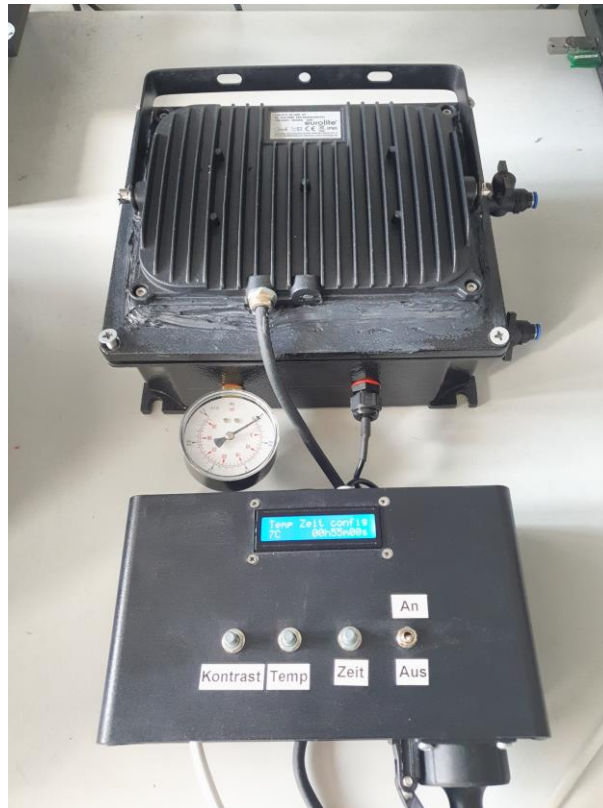
Figure 2.21: An exposure system for the application of refractive index references based on UV-curing polymers has been developed. The system comprises two boxes: the upper box, which can be evacuated, is equipped with a UV lamp, and the second box contains the control electronics. These control electronics switch off the light source when the exposure time is reached or when the maximum permissible temperature is reached. The system is designed to cure polymers in a protective atmosphere and at a defined maximum temperature.
