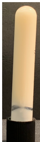
Fig. C.6.1. Viscoelastic emulsion of silicon oil M20 in a nematic gel, initially containing 20 wt% surfactant with R(C_{18:1}E_2CH_2COOH) = 0.655 . The emulsion contains 53 wt% silicon oil, 9.4 wt% surfactant, and 37.6 wt% water. The emulsion was prepared by adding silicon oil and thoroughly mixing by shaking by hand and vortex mixing. Birefringence could not be checked due to strong turbidity, but the viscoelastic gel-like behavior suggests that the nematic phase stayed intact.
