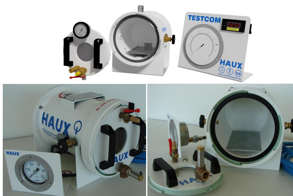
Figure 9. The HAUX Testcom 200/2 pressure chamber used to treat the samples (graphic provided by the Haux-Life-support GmbH).
