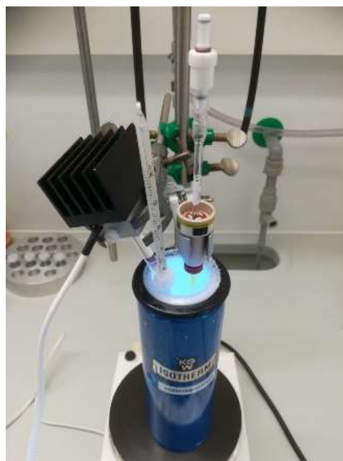
Figure S1. Ex situ illumination setup of NMR samples.
