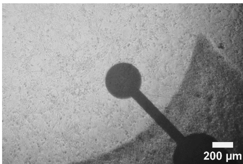
Figure 7. Phase contrast micrograph of CHO K1 cells on a 96W1E+ electrode array. The image was taken with a 4x objective at the Nikon Diaphot microscope.
