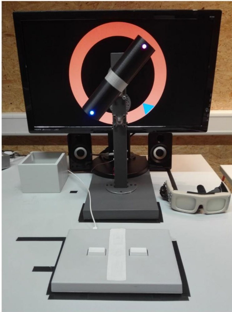
Fig. 2. Display of the RPMC Setup and exemplary solutions to trials solved according to the rule- (exemplary instruction: “If the arrow is green, then I place my thumb on the side of the dowel with the green dot.”) (b) and the plan-based (c) approach (instruction: “I will carry out the movement as comfortably as possible”). (a) Picture of the RPMC setup, including the custom-built turning apparatus in front of the computer screen, response pad (front and center) and shutter goggles (right); adapted from Stoll, et al. 6 . (b) Picture of an RPMC trial which has been solved according to the rule-based approach with a pronated grasp: participants follow the if-then rule. (c) Picture of an RPMC trial which has been solved according to the plan-based approach with a supinated grasp: participants prospectively plan the movement and select a grip that allows them to perform the movement as comfortably as possible.
