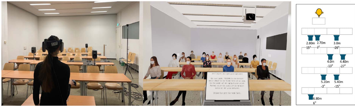
Figure 4. Setup of eye-tracking-paradigm. On the left, the position of participants and loudspeakers (in block 1) in the room are shown. In the middle, a visual virtual room with the eye-tracking task for sound source localization is depicted (participants had to look at the perceived sound source). On the right: source and listener positions.
