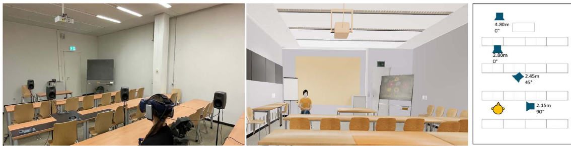
Figure 3. Setup of placement paradigm. On the left: Position of participant and loudspeakers in the room. In the middle: Placement task (Agent had to be placed at perceived sound source). On the right: Source and listener positions.
