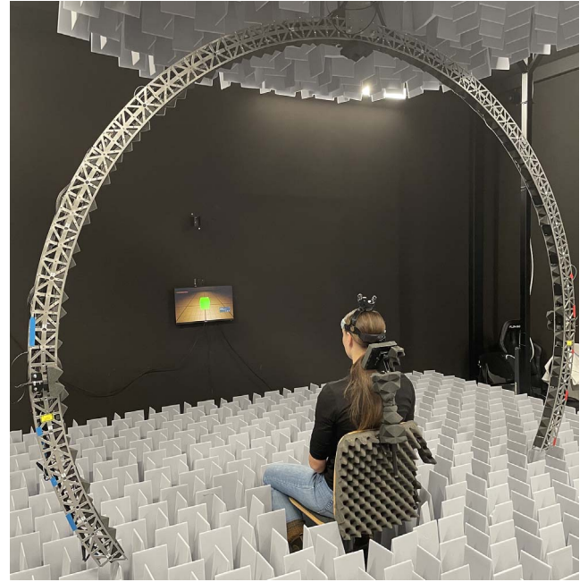
Figure 1. Auditory measurement system of individual and generic (HATS) head-related impulse responses (HRIRs).
