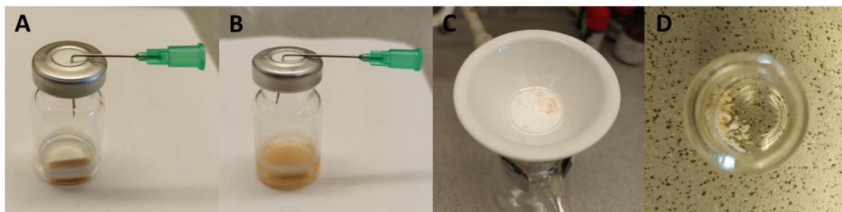
Figure S4. Reaction of 1a . A : reaction mixture before irradiation. B : reaction mixture after 3 h irradiation. C : Filtered product. D : Isolated product.
