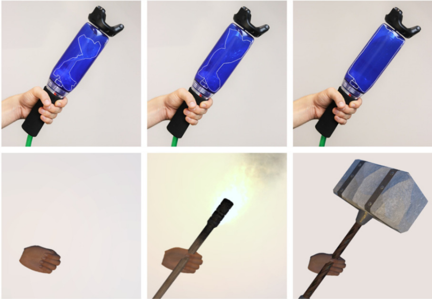
Figure 7: PumpVR at three different weight levels and exemplary virtual objects that these can represent Source: Own representation based on Kalus et al., 2023b: 4
