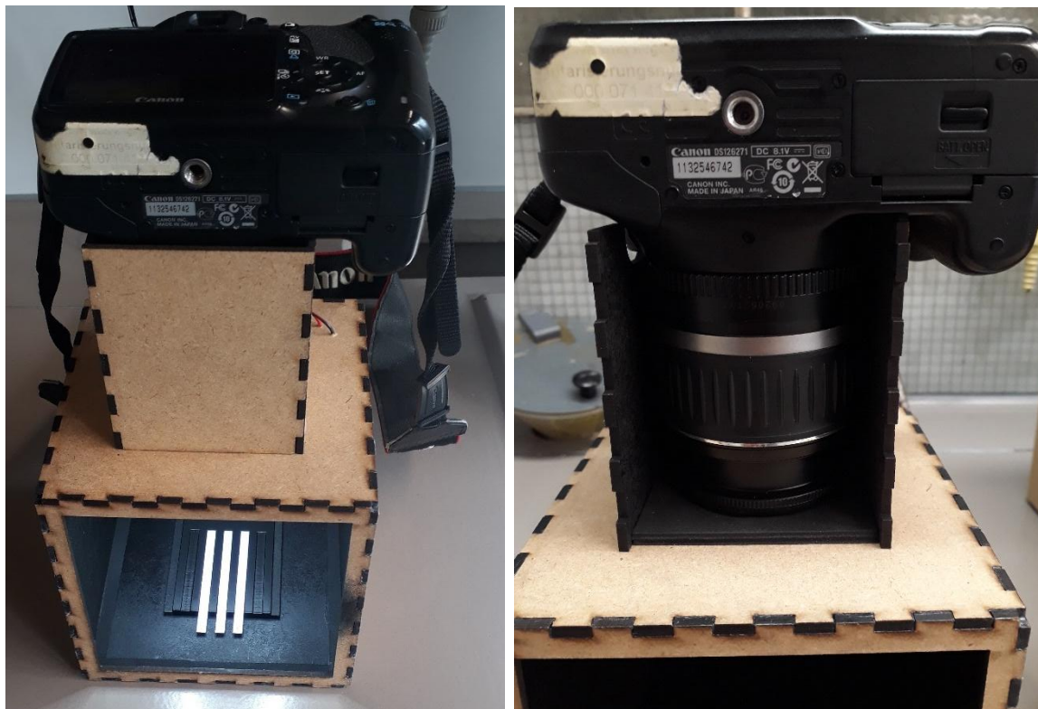
Figure S1: Pictures of the photo box in the opened state. A front cover is added to ensure that no light can penetrate from the outside during imaging.
