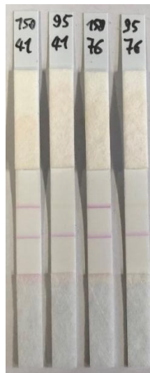
Figure S20: Test strips (1-4 from left to right) run with sera no. 41 (strips 1 and 2) and 76 (strips 3 and 4) from the serum panel previously tested for binding antibodies against SARS-CoV-2 RBD using the recomLine SARS-CoV-2 IgG assay. Strips 1 and 3 contained a streptavidin test line and <anti-FITC> control line on CN150 membrane. Strips 2 and 4 contained a streptavidin test line and FITC control line on CN95 membrane.
