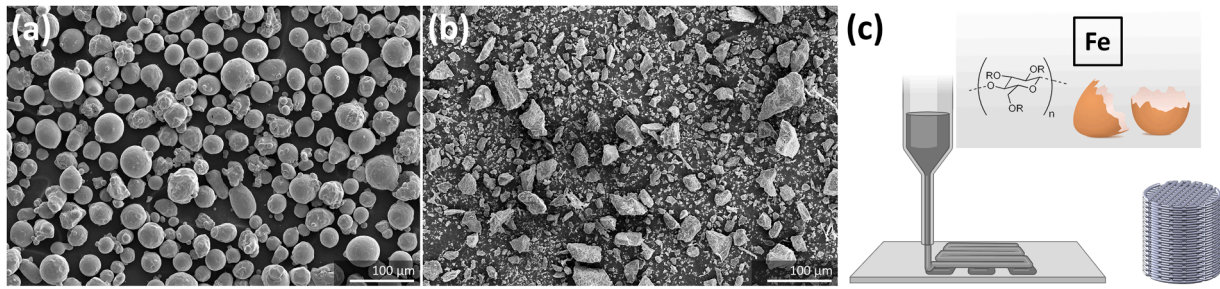
Fig. 1. The morphologies of the (a) Fe and (b) eggshell powders. (c) A schematic illustration of direct ink writing (DIW) of the Fe-eggshell ink and the cylindrical porous scaffold design.
