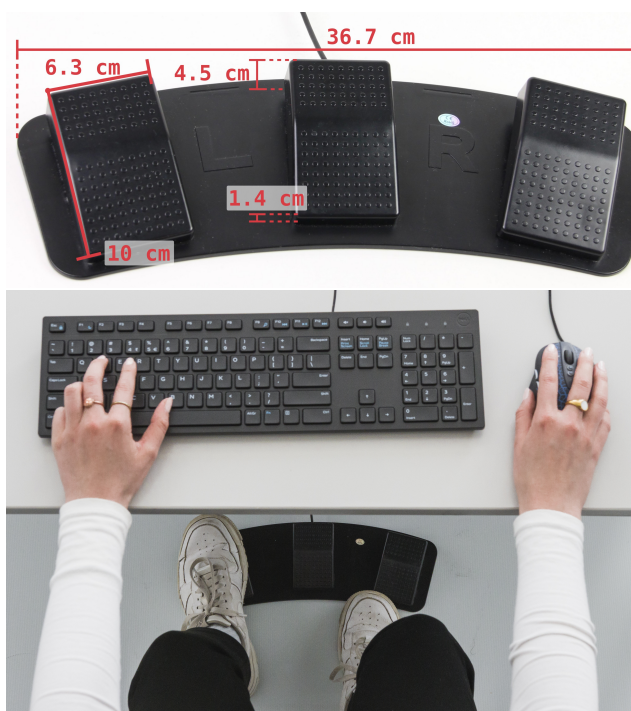
Figure 1: Top: the footswitch used in our user study. It consists of three pedals, each of which triggers a key event on the host computer. Bottom: footswitch used simultaneously with keyboard and mouse.
