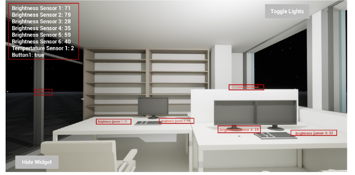
Fig. 4. Screenshot of the Living Lab rendered inside UE5 with embedded sensor readings; the Toggle Lights button allows turning on/off the light in the actual office space. Red boxes display sensor readings.
