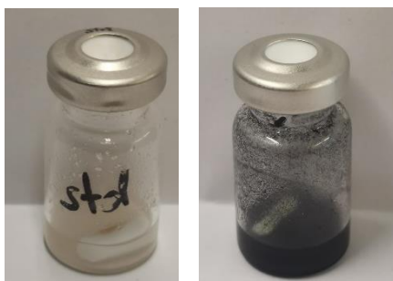
Figure 3.5: Pictures of the reaction mixture in a 5 mL crimp-cap vial before the reaction (left) and after irradiation (right).
