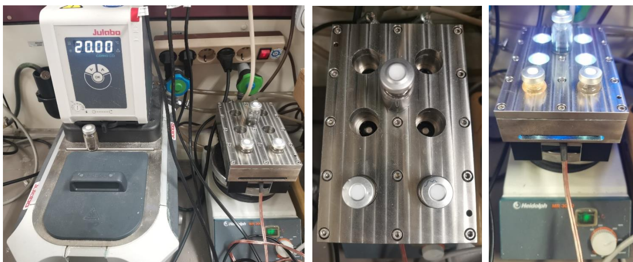
Figure 3.2: Pictures of the photosetup used for reactions run in 365 nm (1.5 W to 2.0 W optical power). General picture of the setup (left), picture from the top of the cooling block looking down to the LED plate (centre) and a sideways picture of the photosetup with lights on (right).
