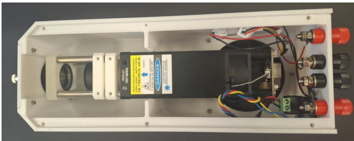
Figure 2.14: Assembled light source, consisting of the laser module, the fiber coupling optics, and connectors for power supply. Components L.2 were 3D printed in this case.
