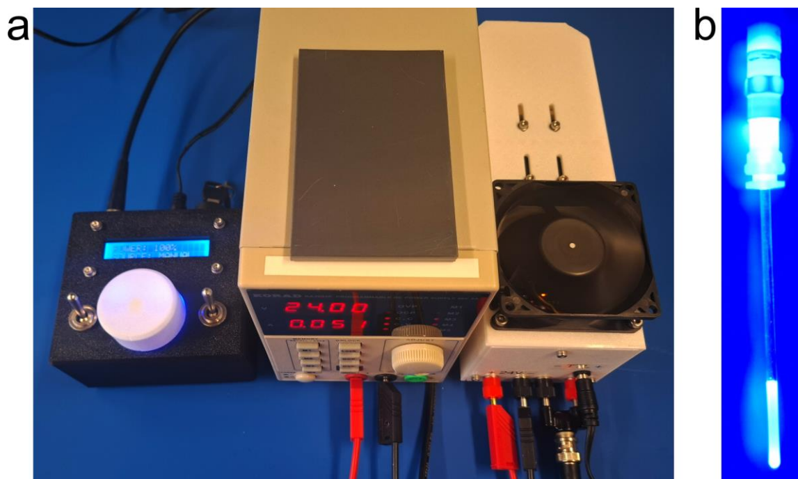
Figure 2.1: Overview of the components of this illumination setup. a) Components outside the magnet: Arduino based control unit, power supply unit, laser module with additional fan and optics. b) Illumination head under operation: Sandblasted medium-walled, NMR-tube and optics on polished fiber end.
