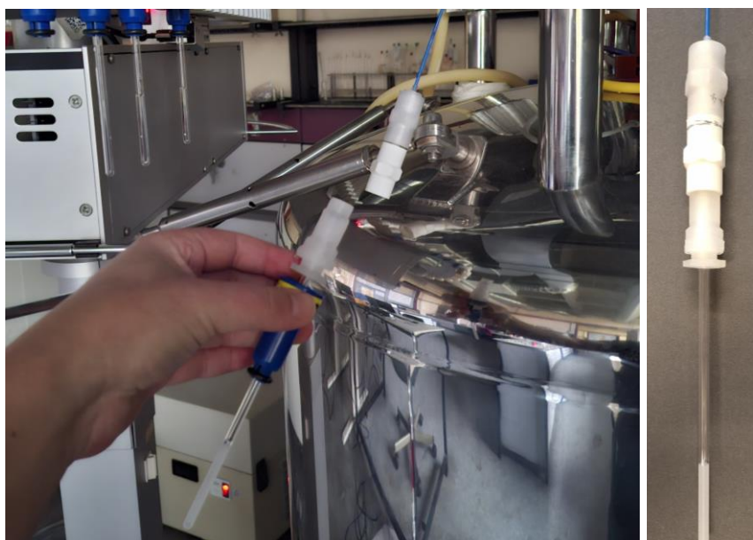
Figure 2.3: Laser setup in use: the sample is connected to the end of the optical fiber with a specially designed, threaded sample cap (“illumination head”), then lowered into the magnet by hand as with other established in-situ illumination methods.
