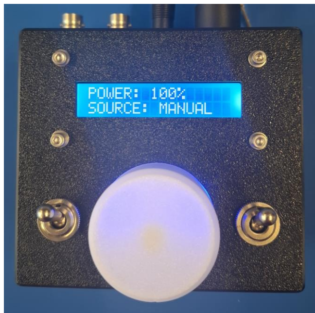
Figure 2.6: Controller of the laser setup: left switch: enable /disable illumination; right switch: select source Spectrometer / manual, knob: adjust illumination power. The current state is written on an LCD.
