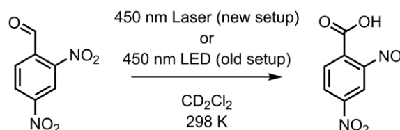
Figure 2.7: Photochemical intramolecular isomerization of 2,4-dinitrobenzaldehyde (DNBA) to 2-nitroso-4-nitrobenzoic acid.
