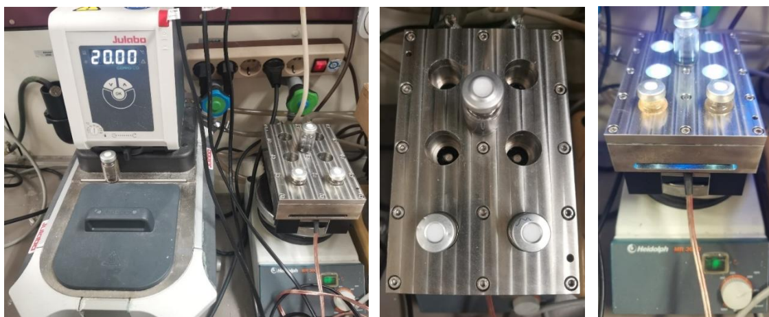
Figure S3.1. Pictures of the photosetup used for reactions run in 365 nm (1.5 W to 2.0 W optical power). General picture of the setup (left), picture from the top of the cooling block looking down to the LED plate (centre) and a sideways picture of the photosetup with lights on (right).
