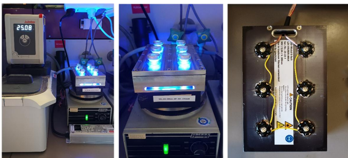
Figure S2.1. Photoreactor setup. A: Thermostat connected to the aluminium cooling block. B: Cooling block and LED on top of stirrer. C: LED module.
