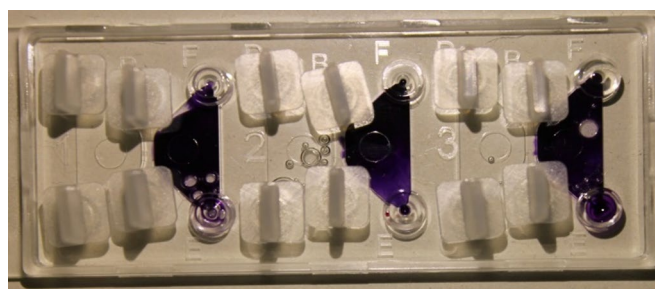
Fig. 4. Composition of the IBIDI \mu -Slide. For better illustration, the right reservoir was stained with blue hematoxylin solution in this figure.
