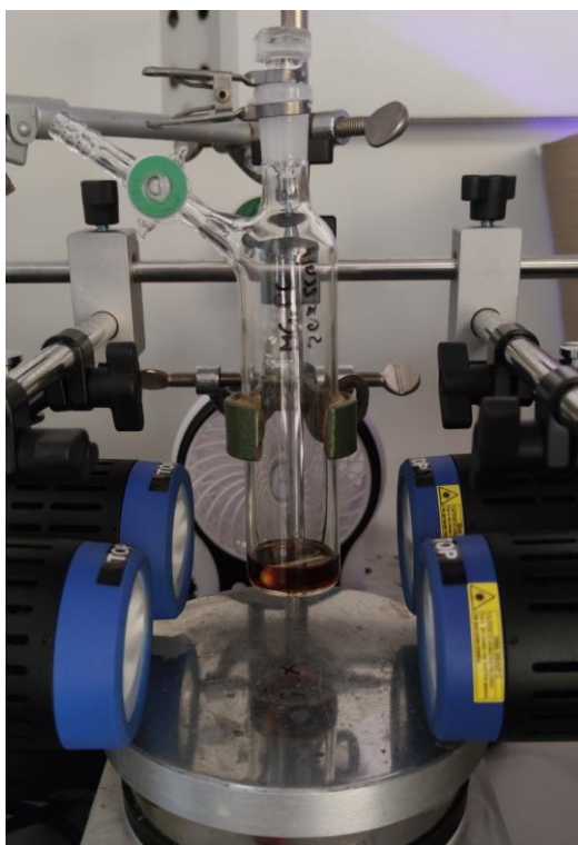
Figure S56. Setup used for photocatalytic reactions at 0.8 mmol scale of \text{P}_4 .
