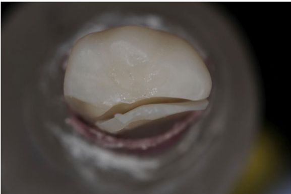
Fig. 8. Typical pattern after fracture testing.
