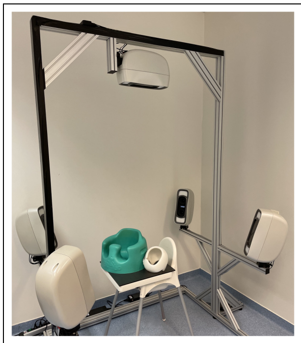
Figure 1. Configuration and calibration of the Vectra M5 360 imaging system, shown in conjunction with a toddler positioning chair and exemplary helmet.
