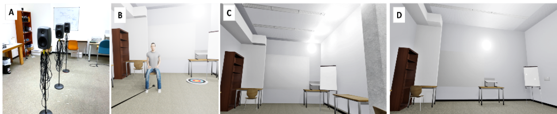
Figure 4: A: Setup of loudspeakers in the experimental room. B: Placement task from participants' view. C: Congruent audiovisual room. D: Incongruent audiovisual room.
