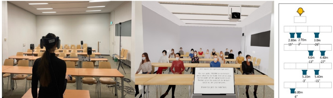
Figure 13: Setup of eye-tracking-paradigm. On the left, the position of participants and loudspeakers (in block 1) in the room are shown. In the middle, a visual virtual room with the eye-tracking task for sound source localization is depicted (participants had to look at the perceived sound source). On the right: source and listener positions.
