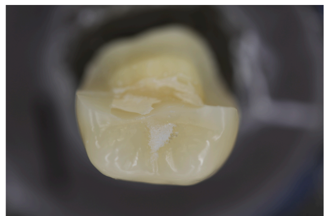
Fig. 3. Typical fracture of the crown (occlusal view, example: CrownX).
